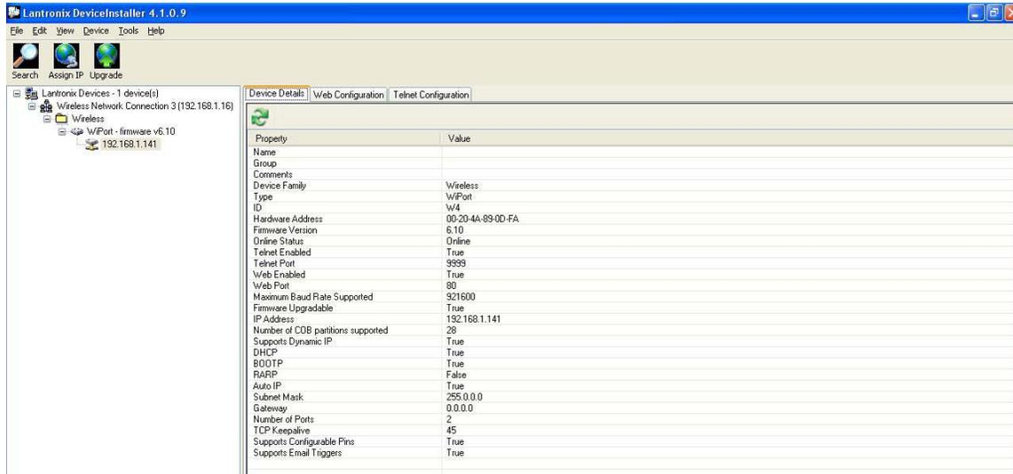
If the device has not yet received an IP address, it will assign itself an address in the 169.254.xxx.xxx address range, with a Class B subnet. Select the device by clicking on the IP, and the option to “Assign IP” will be available on the top menu.
